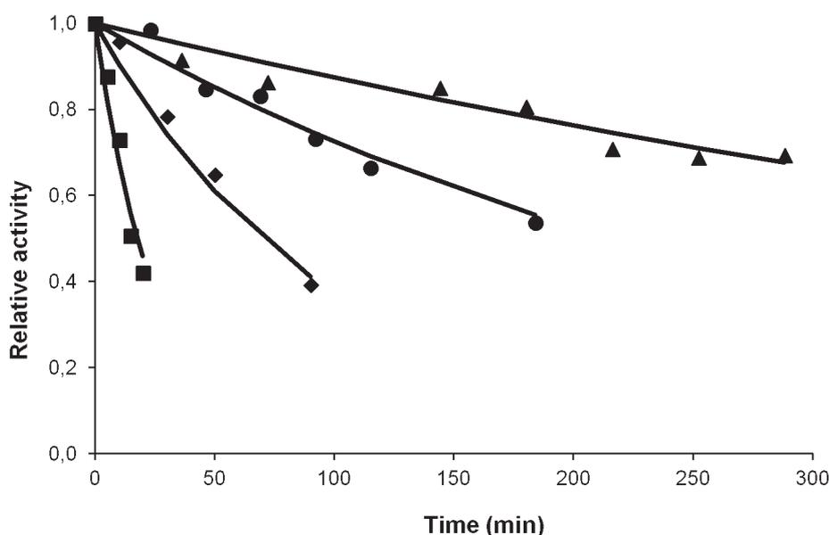
**Fig. 1.** Thermal inactivation of immobilized glucose isomerase in 2.5 mol dm<sup>-3</sup> glucose solution: 83 °C (▲), 86 °C (●), 90 °C (◆), 95 °C (■).
