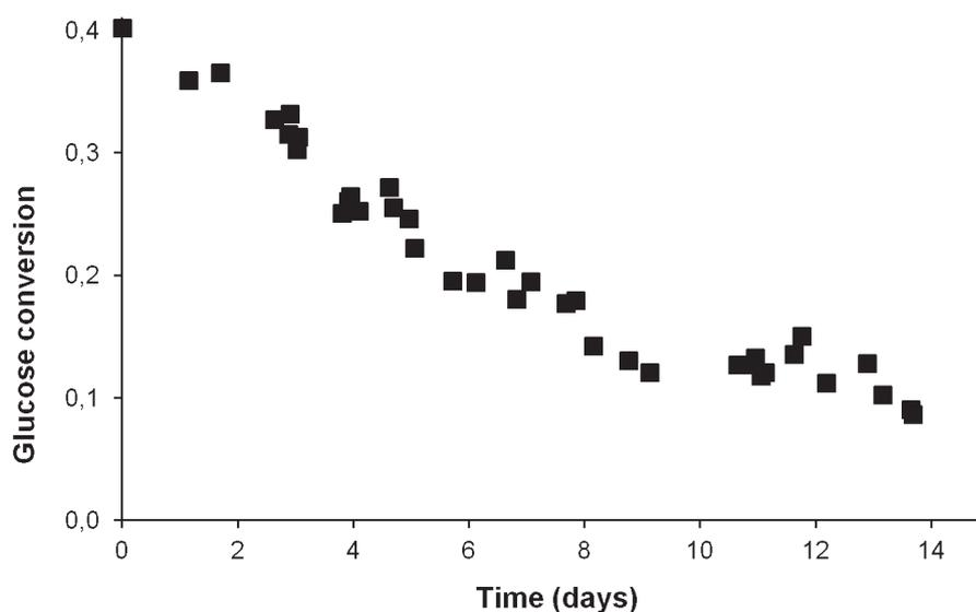
**Fig. 3.** Operational stability of glucose isomerase in a packed-bed reactor at 65 °C. Outlet glucose conversion was measured at the constant flowrate of 2.5 mol dm<sup>-3</sup> glucose feed solution.
