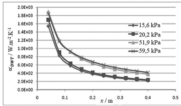
**Fig. 3.** Heat transfer coefficients  $\alpha_{DWT}$  of Dowtherm A along the vertical tube.
