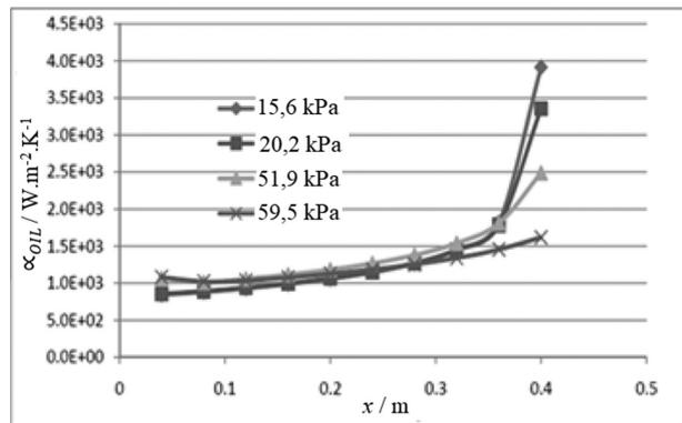
**Fig. 4.** Heat transfer coefficients  $\alpha_{OIL}$  of oil along the vertical tube.
