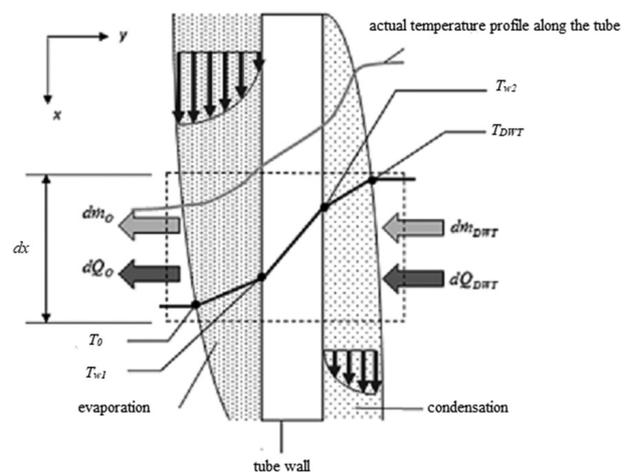
**Fig. 2.** Temperature profile along the vertical tube.
