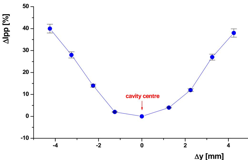
Fig. 3. Variation of the change of the normalised experimentally observed peak-to-peak height of the first-derivative EPR signal,  $\Delta I_{pp}$  [%], on the shift of the sample centre along the cavity y-axis,  $\Delta y$ , out of the centre of the single  $TE_{102}$  rectangular cavity. The averaged values are from five independent measurements. The averaged  $I_{pp}$  value of the correct, concentrically positioned thin cylindrical sample was postulated to be 100 %.
