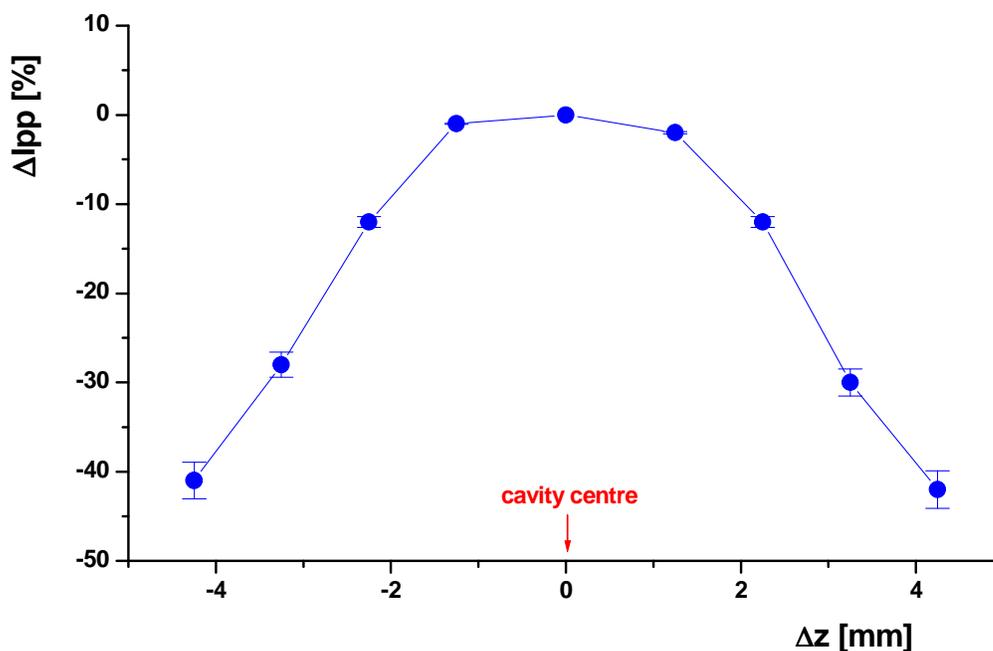
Fig. 2. Variation of the change of the normalised experimentally observed peak-to-peak height of the first-derivative EPR signal,  $\Delta I_{pp}$  [%], on the shift of the sample centre along the cavity  $z$ -axis,  $\Delta z$ , out of the centre of the single  $TE_{102}$  rectangular cavity. The averaged values are from five independent measurements. The averaged  $I_{pp}$  value of the correct, concentrically positioned thin cylindrical sample was postulated to be 100 %.
