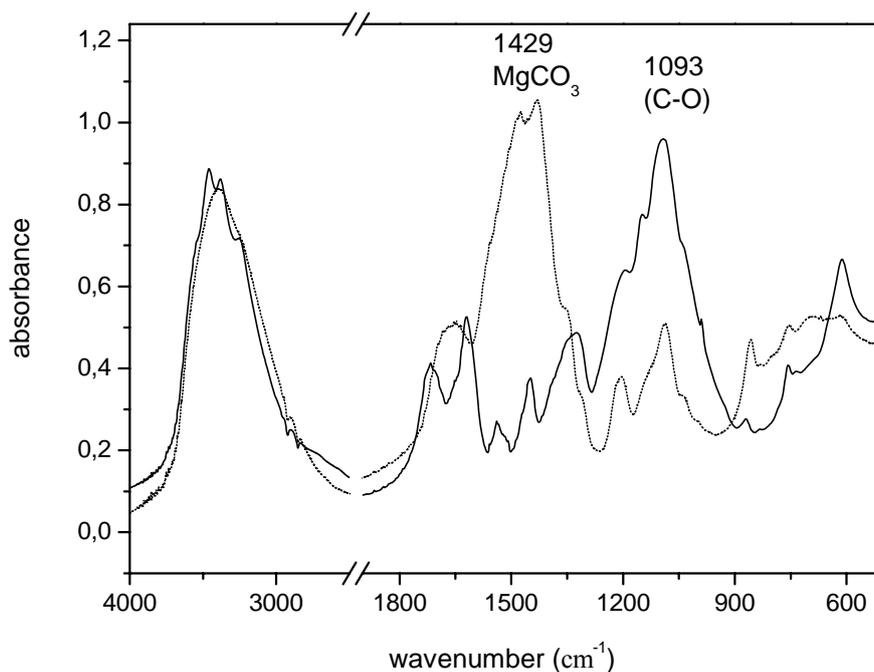
Fig. 10. FTIR spectra of iron gall ink (black line) and iron gall ink with MMMK (dot line) in pellet.
