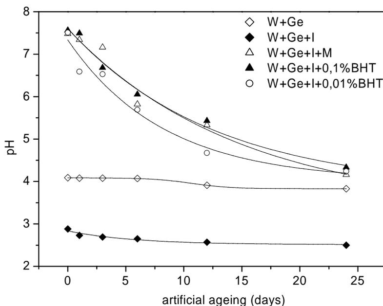
Fig. 4. Dependence of the pH on the ageing time for wet ageing at 80°C, 50% RH for ink samples
