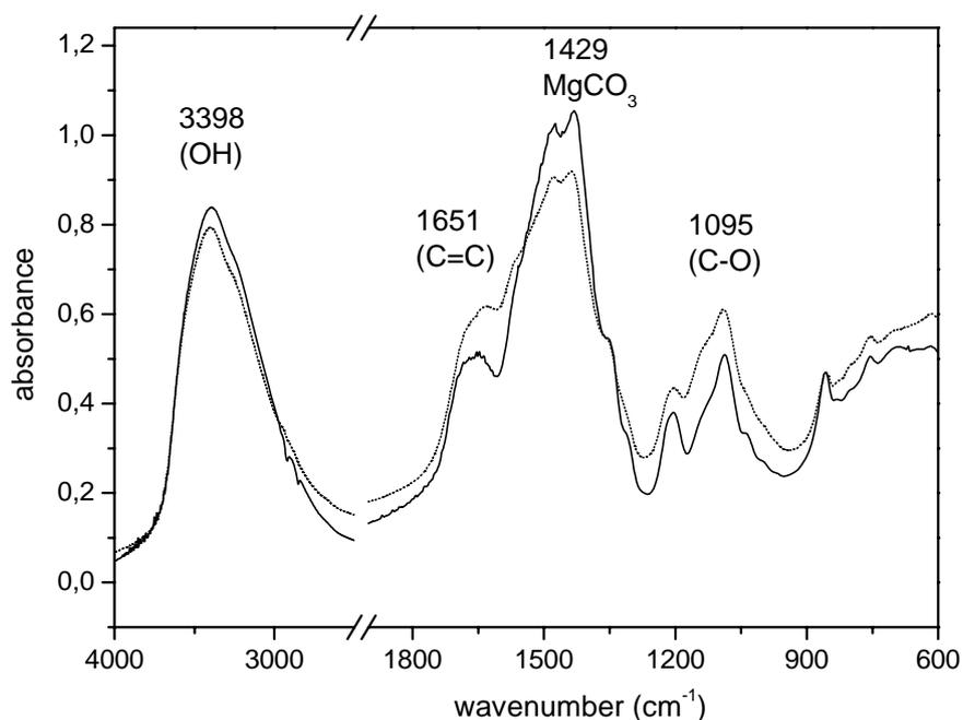
Fig. 11. FTIR spectra of iron gall ink with MMMK in pellet. Black line: no ageing, dot line: aged 3 days
