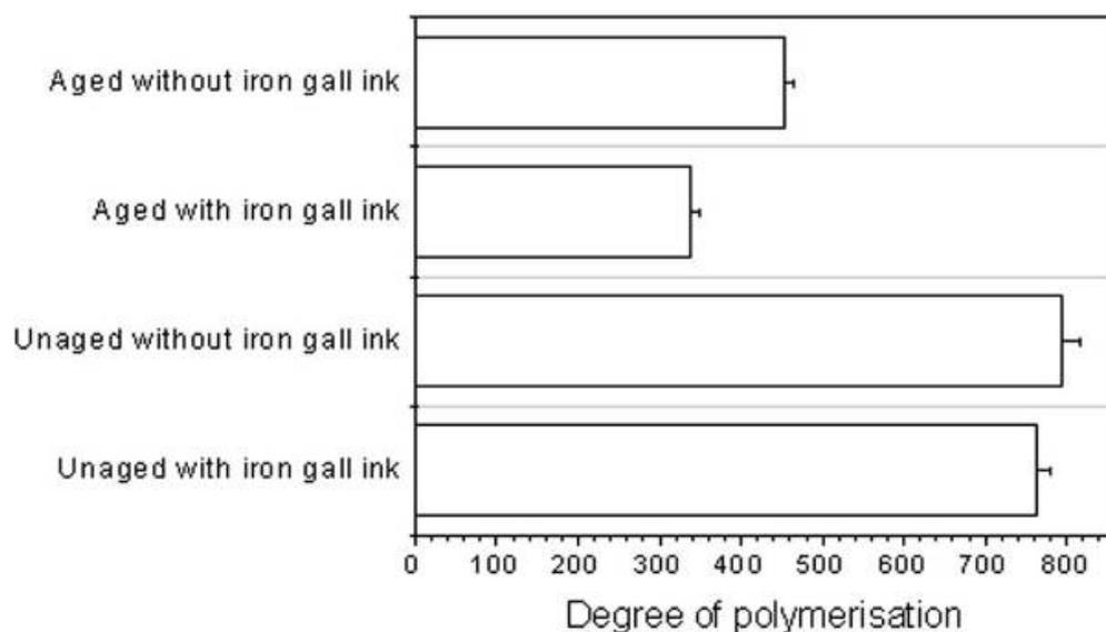
Fig.3. The comparison of degree of polymerisation in aged and unaged paper with or without ink line
