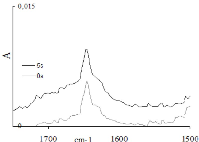
Fig.7 ATR-FTIR spectrum of untreated (0s) and plasma treated (5s) PP films
