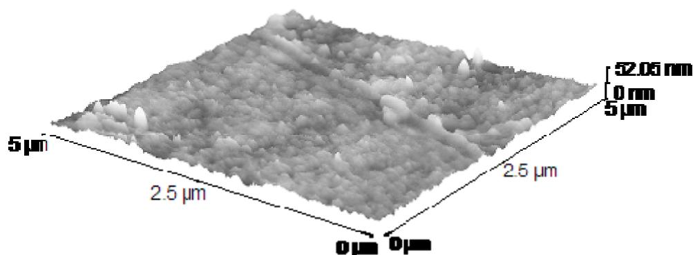
Fig.5 AFM image of the untreated film, RSM= 3.1nm
