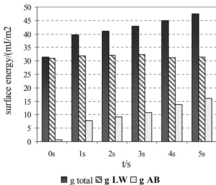
Fig.3 Influence of the time of plasma treatment on the surface energy
