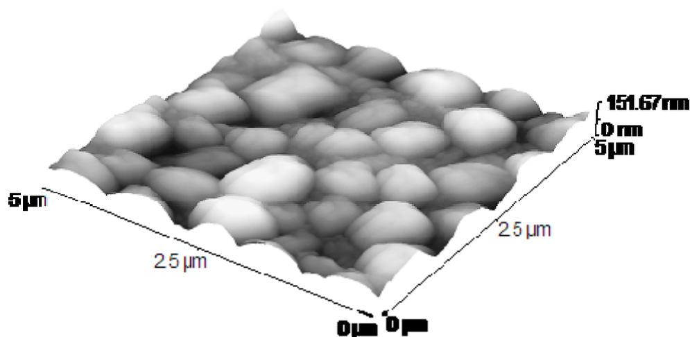
Fig.6 AFM image of the 5s plasma treated film, RSM= 24nm
