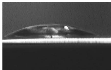
Fig.2 A drop of water on the PP film plasma **after** plasma treatment (5s)
