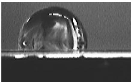
Fig.1 A drop of water on the PP film **before** treatment
