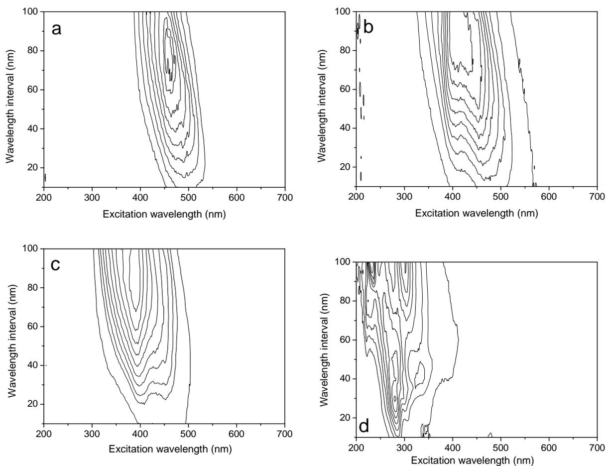
Fig. 2 Contour plots of total synchronous fluorescence spectra of brandy (a), whisky (b), slivovice (c), and juniper spirit (d) samples. Contours join the points of equal fluorescence intensity.
