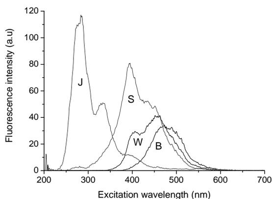
Fig. 3 Synchronous fluorescence spectra of brandy (B), whisky (W), slivovice (S), and juniper spirit (J) recorded at wavelength interval 40 nm.
