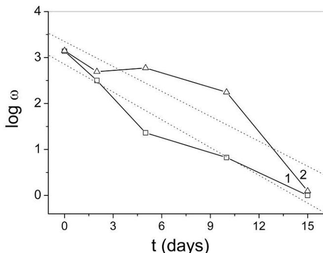
Fig.3. Effect of ageing time ( $t$ , days) on logarithm of folding endurance ( $\omega$ , double folds): 1 - non-treated newsprint paper, 2 - newsprint paper treated by carbonated magnesium propylate dissolved in heptafluoropropane
