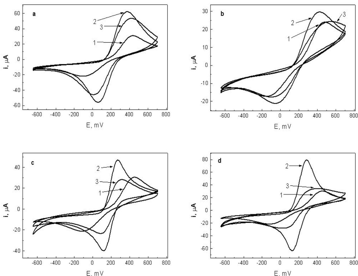
Fig. 2. Comparison of cyclic voltammograms of  $[\text{Fe}(\text{CN})_6]^{3-/4-}$  obtained at SPCE (1), CHIT-CNT/SPCE (2) and DNA/CHIT-CNT/SPCE (3) ((a) without CNT, (b) SWNT, (c) MWNT, (d) SWNT-COOH). Conditions:  $1.10^{-3} \text{ mol dm}^{-3}$   $[\text{Fe}(\text{CN})_6]^{3-/4-}$ ,  $0.1 \text{ mol dm}^{-3}$  PBS, scan rate  $50 \text{ mV s}^{-1}$ .
