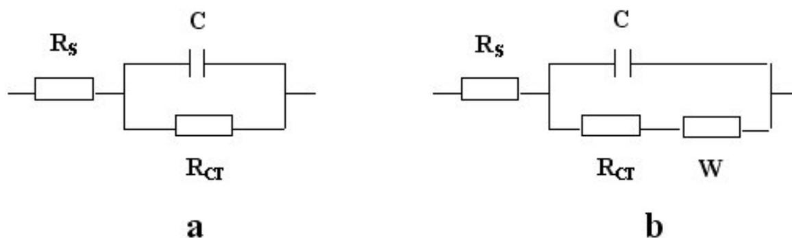
Fig. 3. Equivalent circuits used for fitting experimental EIS data.
